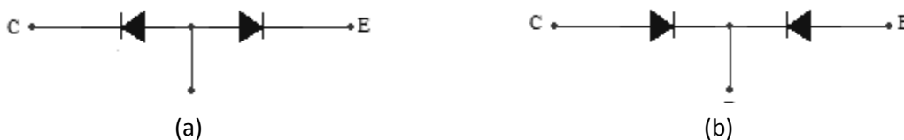
Figure-7: Diode equivalent of a NPN (a) and a PNP (b) Transistor
