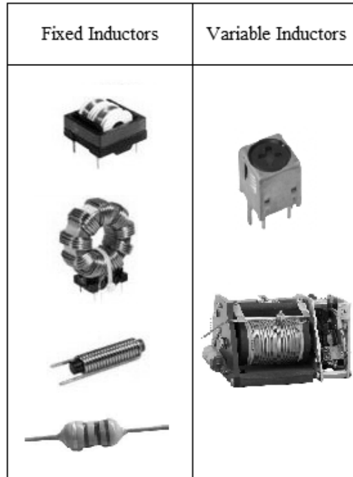
Figure-6: Some real inductors
