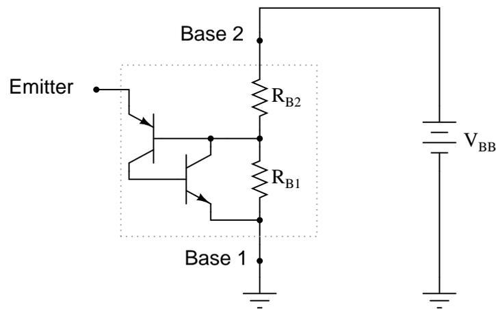
How much voltage, and of what polarity, must be applied to the emitter terminal of the UJT to turn it on? Write an equation solving for the magnitude of this triggering voltage (symbolized as  $V_P$ ), given  $R_{B1}$ ,  $R_{B2}$ , and  $V_{BB}$ .
