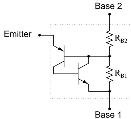
When the two base terminals of a UJT are connected across a source of DC voltage, the two base resistances ( $R_{B1}$  and  $R_{B2}$ ) form a voltage divider, splitting the applied voltage into lesser portions:
