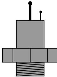
With no test instrument other than a simple continuity tester (battery and light bulb connected in series, with two test leads), how could you determine the identities of the three terminals on this SCR?
