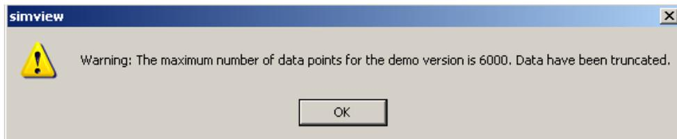
Increasing the **Print step** in Simulation Control may overcome this problem with the price of lower resolution of the waveform.
