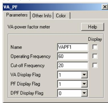
Operating frequency is set according to the frequency of ac voltage source.
