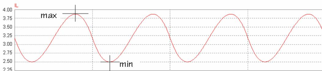
Obtain maximum & minimum values of waveform. The difference between max & min is the peak-peak ripple value. Find peak-peak ripple of Vo and IL from simulation.
